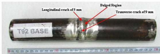
Fig. 11. Visual inspection of failed base specimen after subjected to thermal fatigue.
