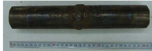
Fig. 4. Weld specimen before subjected to thermal fatigue.
