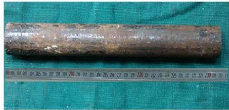
Fig. 1. T-92 base tube before subjected to thermal fatigue.
