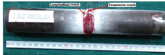
Fig. 14. Liquid penetrate examination of failed weld specimen.
